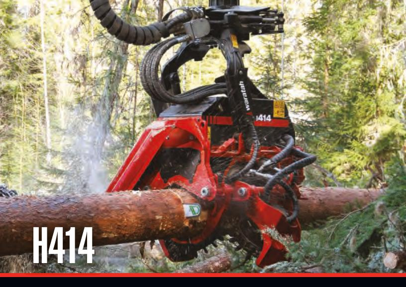
Whether you're harvesting early thinnings or regeneration cuts, the H414 boasts excellent maneuverability and drive power with a relatively compact size. This productive mid-sized harvesting head makes short work of even the most challenging stands.
